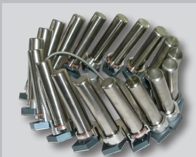
holder with 32 x 100ml beakers with or without dosing nipple
