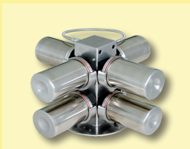
holder with 8 x 500ml beakers for wash tests
