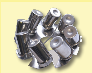
holder with 12 x 500ml beakers with or without dosing nipple
