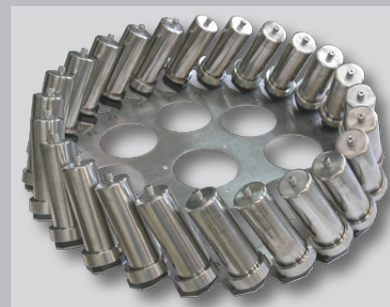
holder with 24 x 200/300ml beakers with or without dosing nipple
