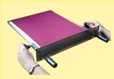
Pin frame adjustable in length: sample is attached on pin border on both sides of the holder, and stretched with 0 to 10 kP.
