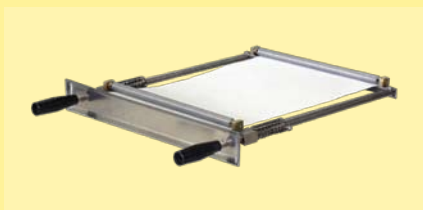
Paper and foil frame: for paper samples and other kind of foils
