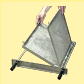
Sieve frame: special holder with two steel nets to keep samples in between, as for example, fibers, tops, paper mass, non-woven, etc.
