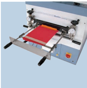
The doctor knife coating followed by drying in controlled hot air.
