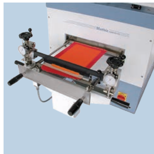
The doctor knife coating followed by drying in controlled hot air.
