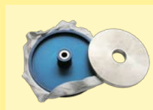
ISO 12945-2 sample holder & 260g load piece
